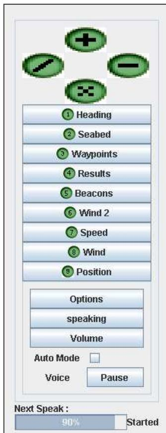
(1) **Heading menu:** surface heading, ground heading, average surface heading and average ground heading;
