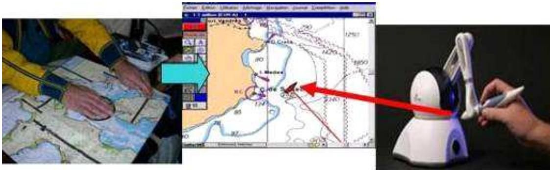
General description : In order to describe Seatouch utilization, it is separated into the six following modules: the map provider part, the haptic part, the sonification part, the vocal part, the simulation part and the NMEA part. All interaction commands are available in a vocal menu using the arrows, enter and backspace keys, or by keyboard shortcuts, and soon by vocal recognition using VOCON 3200 software.
