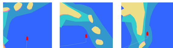
Picture 7: The Heading mode of SeaTouch : while changing boat directions, its position and orientation in the workspace stay stable but the map moves.
